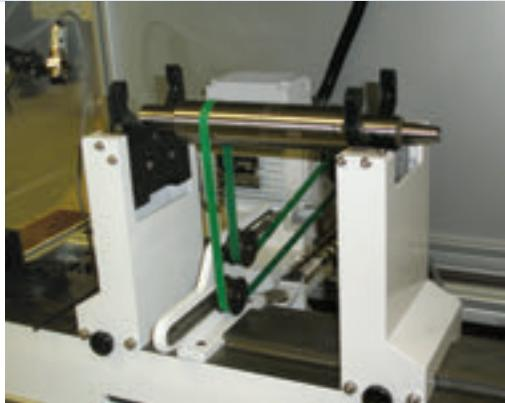
As both cradles are 'floating', both columns have a cradle lock, so one can be fixed whilst the other is being used to give out-of-balance readings.
