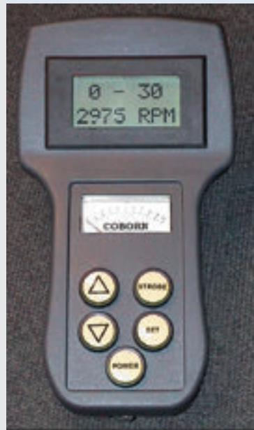
The very successful PB1 has been superseded by the updated PB2. The physical characteristics are exactly the same. The internal design has been simplified and obsolete or non conformity components removed.
