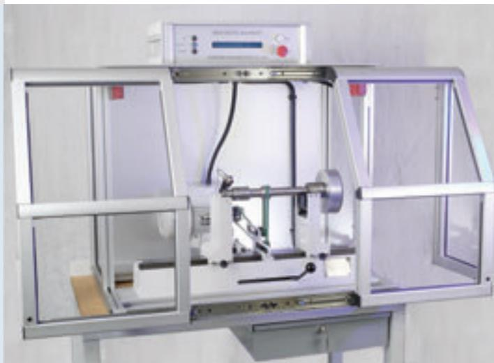
The DB1 and DB2's are single plane static balancing machines.
